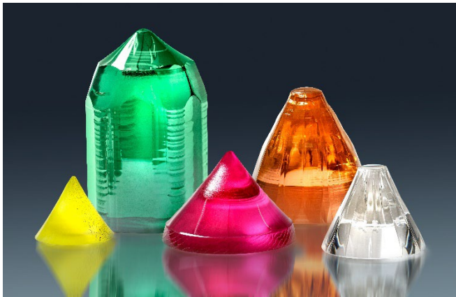
Fig. 1 Various oxide laser crystals with different active dopants (rare-earth elements and transition metals).
