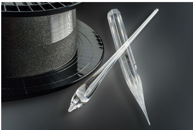
Fig. 2 Octagonal fiber preform, glass gobs from the beginning of the fiber drawing process and active laser fiber on carrier roller.
