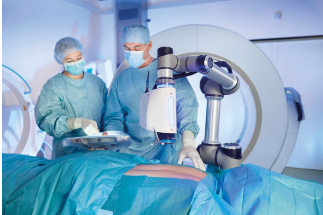
Picture 4: High-risk: Surgical opening of the vertebral body. The robotically assisted, hand-guided laser surgery system developed at Fraunhofer ILT is intended to replace mechanical high-speed milling and minimize surgical risks. Talk to our experts at MedtecLIVE! © Fraunhofer ILT, Aachen, Germany / Ralf Baumgarten.
