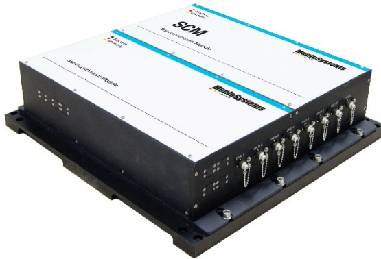
Figure 2: The SCM supercontinuum module for up to 8 beat signals
