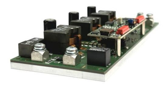
Caption: The compact LDDP-30-125 high-power laser diode driver from SCHULZ-ELECTRONIC is the smallest buck/boost converter in its performance class.
