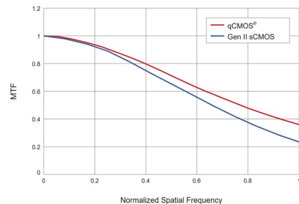
Modulation Transfer Function (MTF) is a type of resolution evaluation. It is the value of how accurately the contrast of an object can be reproduced.
