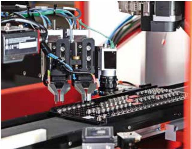
Multiple device trays and feeders increase the throughput and allow for the automated processing of large quantities. Alternatively, an inline configuration with conveyor belts provides a seamless production flow.
