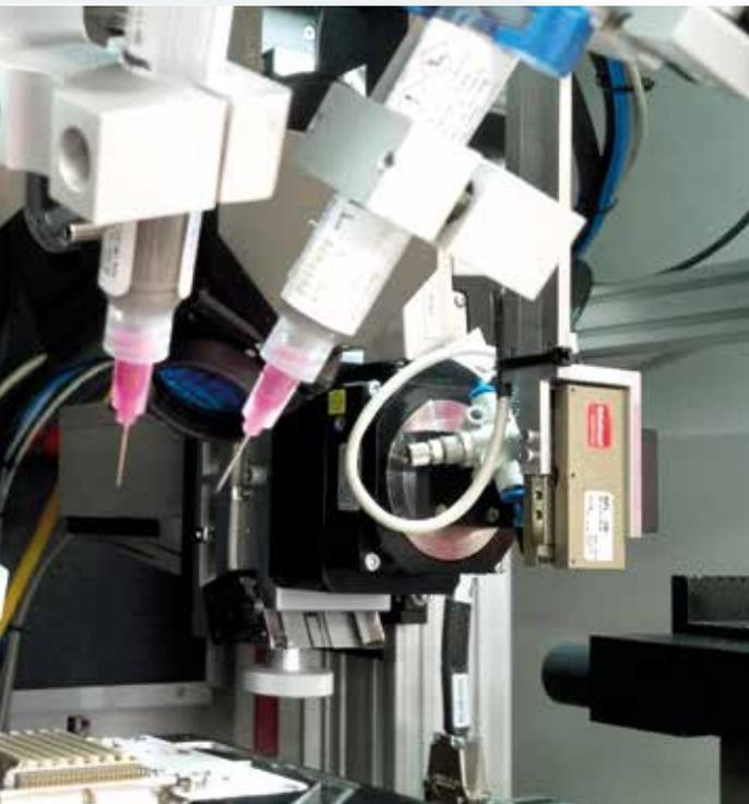
Various assembly techniques can be combined in one station, such as laser welding, laser soldering and epoxy gluing. Exchangeable device trays improve the versatile micro assembly in various batch processes.
