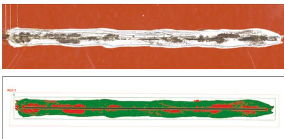
Automatic evaluation of corrosion and delamination using the color scanner system „Corrosion Inspector“. The Scanner detects red rust areas and measures the effected area as well as the delamination area. The scribe area is subtracted from both areas.
