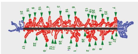
Automated evaluation of various corrosion parameters of different scribe pattern. Among other things, the infiltration area, the average infiltration width, length and number of threads are measured.
