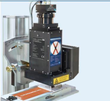
Measurement and evaluation of corrosion phenomena on coated test panels 10
