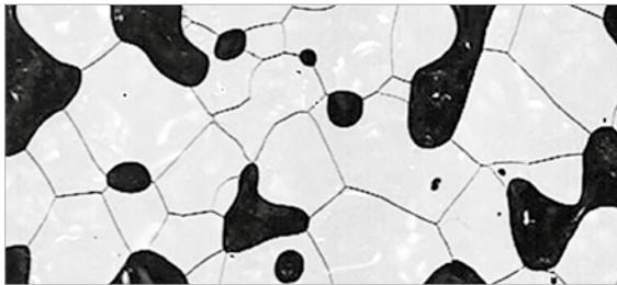
Scan of an ice core from a depth of 60 m under Antarctica. The light granular structure and dark gas bubbles are clearly discernable.
