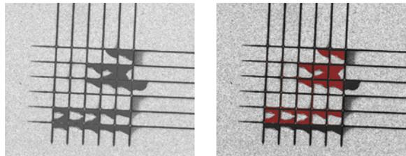
Cross-cut test, delaminated areas are marked in red.
