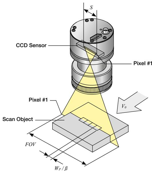
The native resolution of an optical line scan camera is defined by the number of pixels – the row of photosensitive elements in the sensor line. Line scan cameras are available with more than 8000 pixels. The resolution of the scanner system is determined by the objective lens chosen and the scale of the image  $\beta'$ , as a function of the ratio of image size (FOV, field of view) to object size S:
