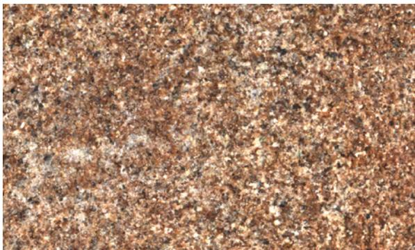
During geological exploration for oil, gas, ores or minerals, a large number of drill core plugs are produced for evaluation. The lateral surfaces of the cores need to be visualized in high quality with subsequent storage of lossless data in digital form.
