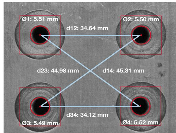
Using the linear scanner system from Schäfter+Kirchhoff, the measurement of distances, dimensions and positions of objects is possible.
