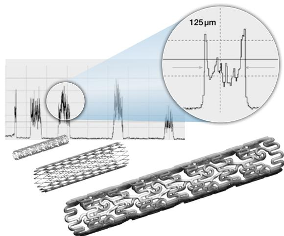
Surface quality and dimensions are detected using a telecentric lens and a line scan camera with integrated bright-field illumination.
