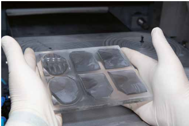
Figure 20: Scanning mirrors during CNC production
