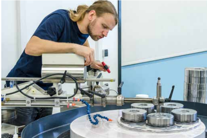
Figure 1: Conventional polishing of plane surfaces
