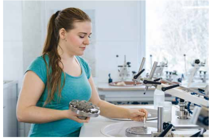
Figure 2: Conventional polishing of spherical optics
