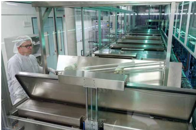
Figure 5: Large optics ultrasonic cleaning process
