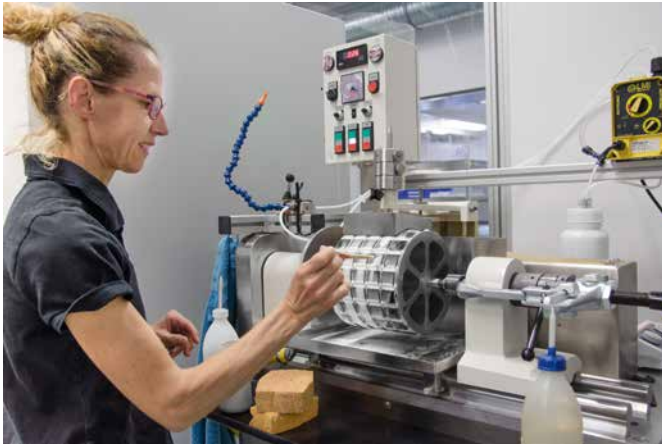
Figure 9: Polishing machine for cylinder optics
