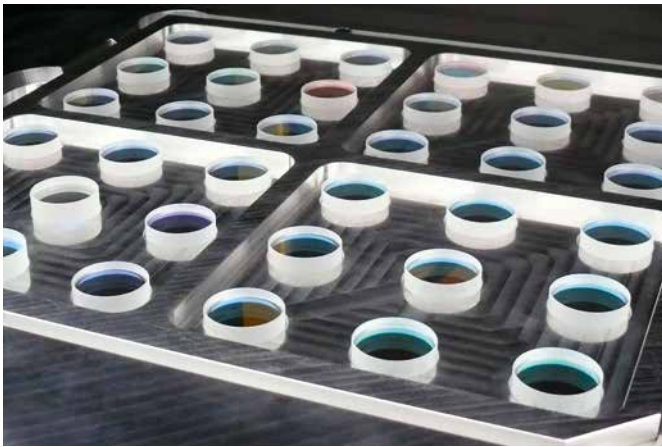
Figure 16: Laser mirrors are placed in a special magazine holder for automated defect inspection at LAYERTEC.
