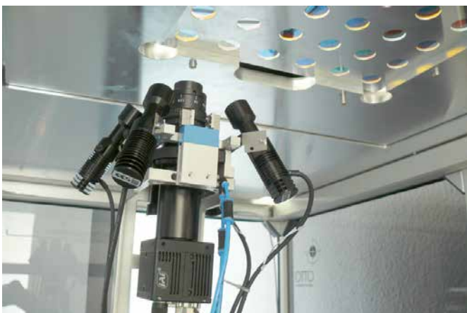
Figure 9: Defect inspection system for optical components
