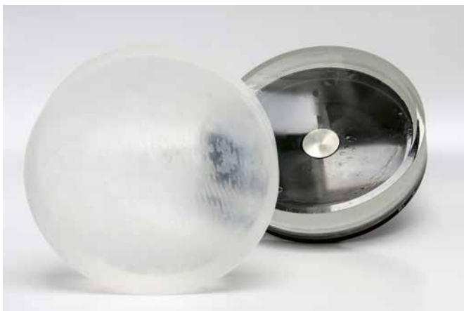
Figure 12: Parabolic substrate in production process, before (l.) and after lapping and polishing (r.)
