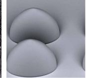
High quality microoptical elements with varying shapes (e.g. freeform) and sizes can be fabricated either on planar substrates or directly on active/ passive devices.
