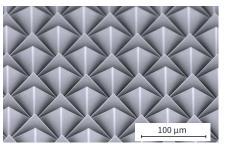
Retro-reflector: Fabrication of high-quality masters used in diverse replication technologies.
