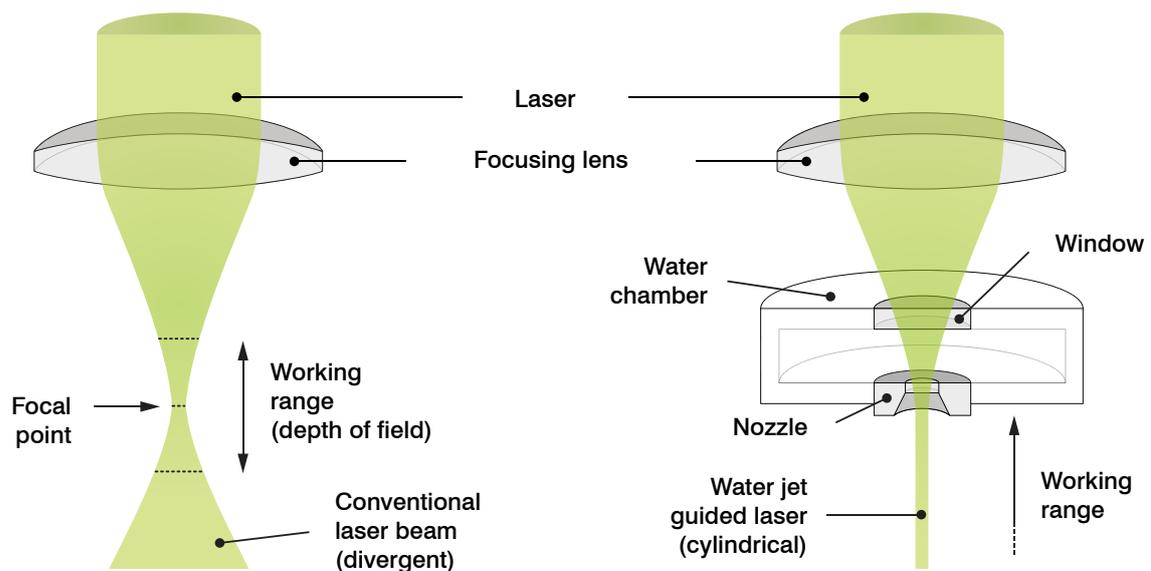
The conventional focused laser beam has a limited working distance of just a few millimetres to even fractions of a millimetre due to beam divergence.
