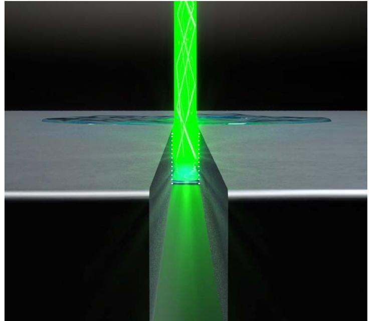
The cutting kerf width ranges from 25 to 120  $\mu\text{m}$ , depending on the nozzle size. The laser energy is always guided to the bottom of the kerf.
