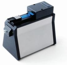
THE CLEAVEMETER 3D<sup>™</sup> is a non-contact interferometer designed for inspecting the end-faces of cleaved or polished optical fibers with cladding diameters of 125 µm to 1200 µm. It gives immediate and precise information on important endface properties such as flatness, perpendicularity, hackles and dust. Based on the NYFORS CLEAVEMETER 2<sup>™</sup> design, in addition to producing sharp fringe patterns it also generates three-dimensional images of the cleaved fiber end.
