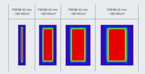
High degree of design freedom for the 'infinitely variable' laser spot – from fine line to largearea irradiation (spot format is predefined in the laser head) – line widths from 40 to 600 mm at 300 mm working distance.
