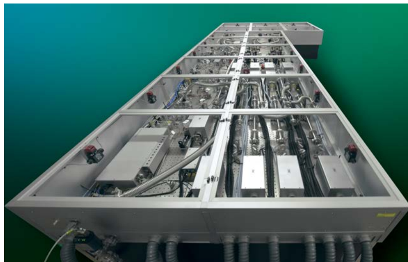
Fig 2. Integrated multi-channel high energy APL pump lasers into OPCPA
