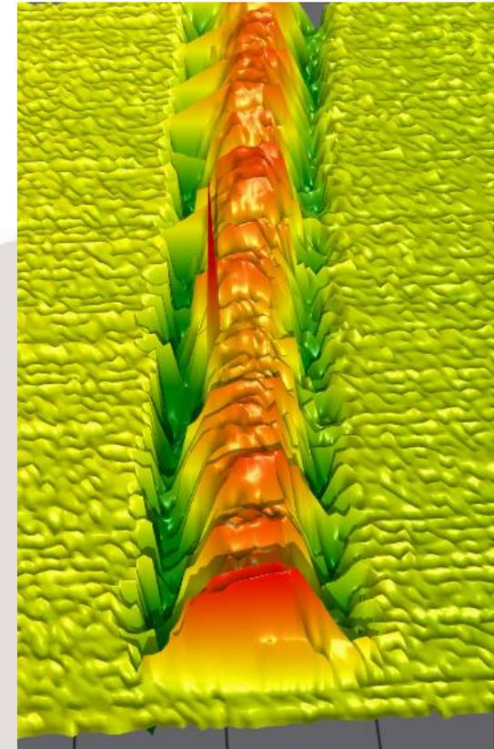
Post-process seam visualization (overlap weld of steel, low-res measurement done online)
