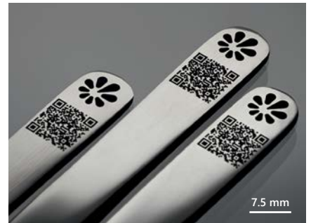
Highly-resistant black marking. Courtesy of FTMC.
