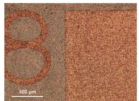
Insulation layer removal from PCB. Courtesy of FTMC.
