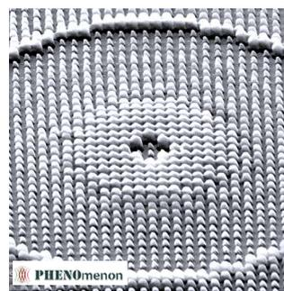
Metastructures with feature sizes below the diffraction limit can be fabricated in a single process step.
