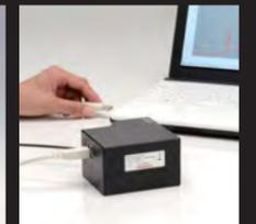
Mini-spectrometer for environmental measurement
