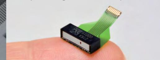
We have developed an ultra-compact grating type spectrometer by using advanced MOEMS (Micro-Opto-Electro-Mechanical Systems) technology to fabricate and combine a CMOS image sensor and grating, etc.
