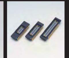
Image sensors for blood tests
