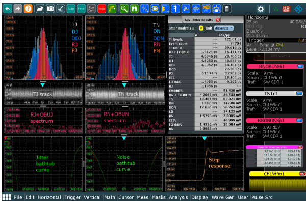
Jitter and noise analysis: displays step response, individual jitter and noise components in histograms, spectrum, synthetic eye diagram and BER bathtub curves.
