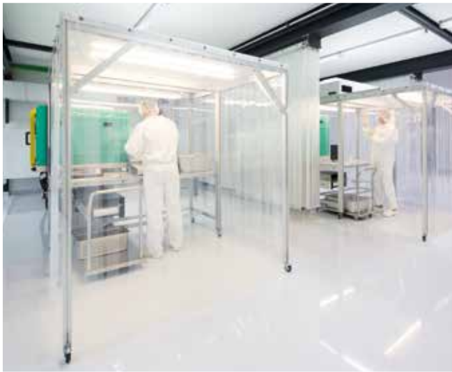
Clean room cell "Soft wall" for injection moulding
